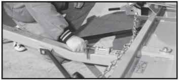
2) Pull locking pin toward the hitch as far as it will go. The wheel platform will tilt back to allow loading.
